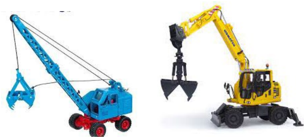
Figure 4-21 Clamshell dragline excavator and a simple excavator having clamshell bucket
