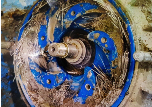
Figure 4-19 Bar screen and a choked impeller
