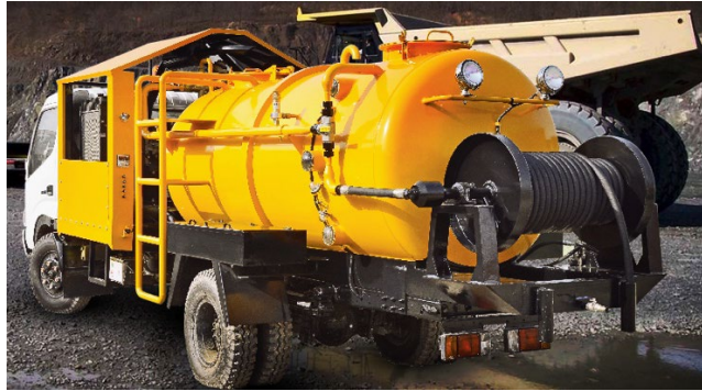
Figure 3-9 Sewer high pressure jetting machine
