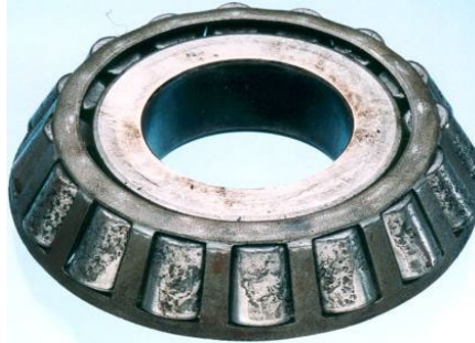
Figure 4-32 Contaminated bearing with water
