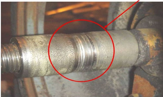
Figure 4-23 Shaft of pump worn out at sleeve due to gland packing
