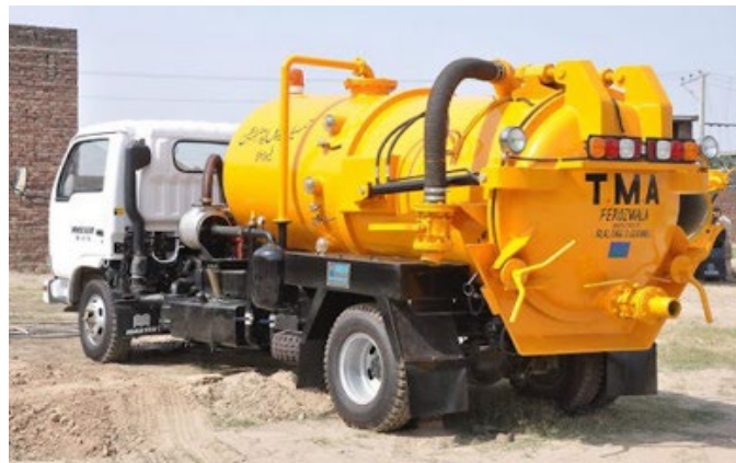
Figure 3-11 Sludge suction machine
